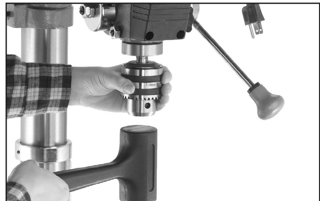
Figure 14. Seating chuck into spindle. (Note retracted jaws.)
